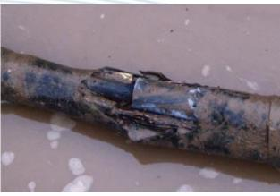
Excavator contact with HV cable
